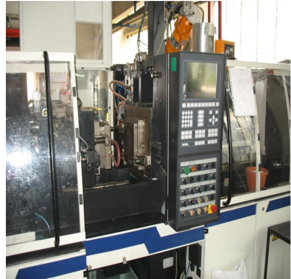
Fig. 4. Injection molding machine ENGEL CC. 100 Type ES 80/50 HL
