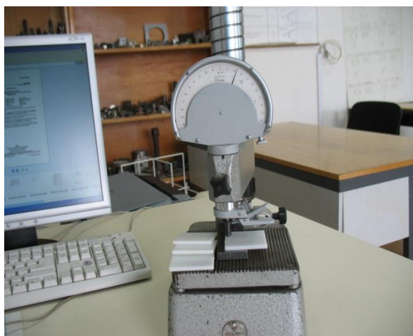
Fig. 7. Warpage measurement with orthotest [5]
